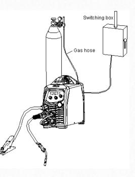
selector into the "+" output terminal of the welding machine, and tighten it clockwise.
