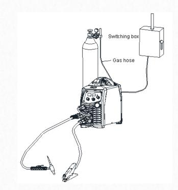
Using valve type torch - No trigger
